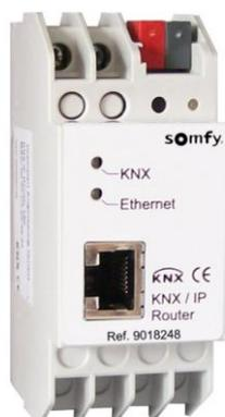
This device works according to the KNXnet/IP specification using the core, the device management, the tunnelling and the routing part. The device supports 5 simultaneous KNXnet/IP tunnelling connections.
